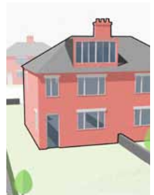
Image showing poorly-designed oversized dormer.
